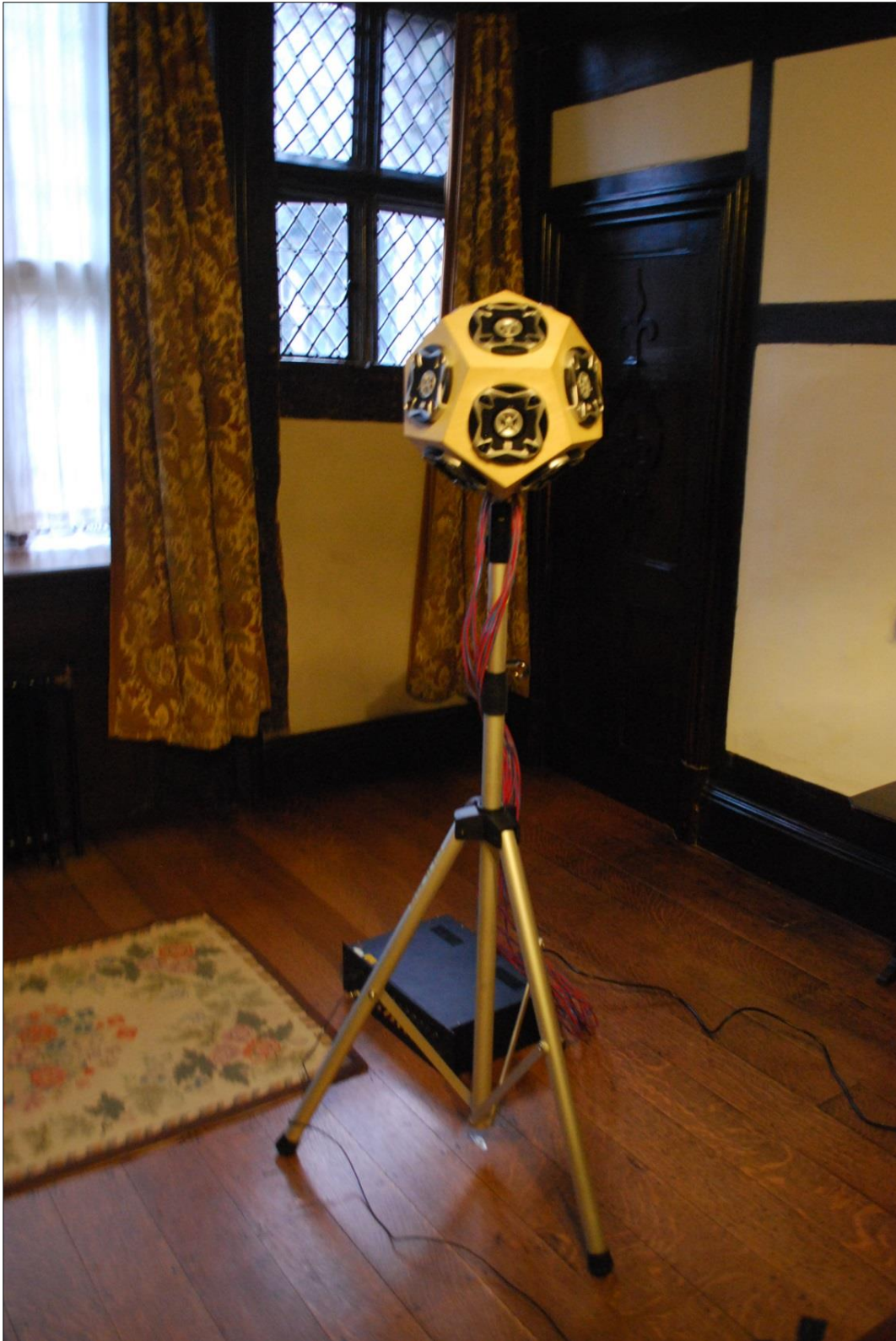
Figure 264: Omnidirectional loudspeaker used in acoustical survey. Each of the black circles is a directional speaker allowing sound to be emitted in “all” directions.
