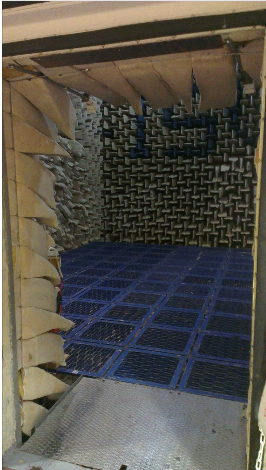
Figure 268: The Anchoic Chamber at University of Southampton. This room does not reverberate; it is a “dead” space. This allows us to record sounds to be used in Auralization or test the quality of instruments to be used in acoustical testing.
