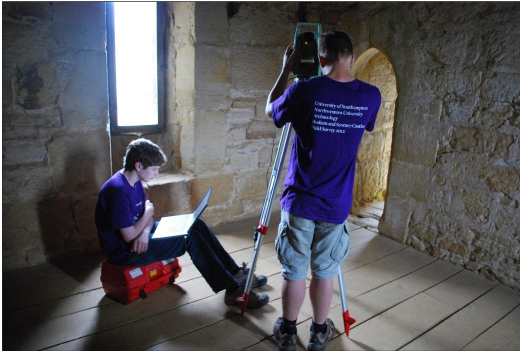
Figure 67: Total Station Connected to Laptop. Survey work being undertaken by Southampton students Ben Culpin and Tom Young in August 2012.
