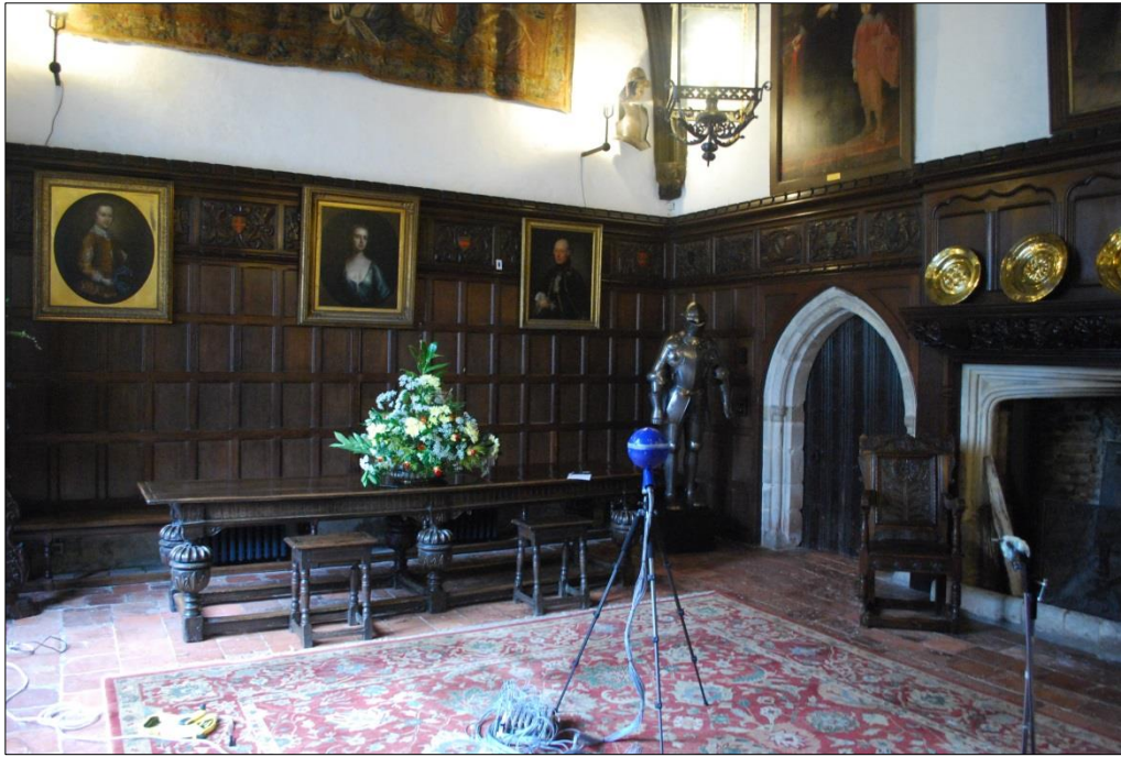
Figure 266: Omnidirectional microphone, this consists of microphones pointing in "all" directions allowing sound to be recorded as it is received from different directions
