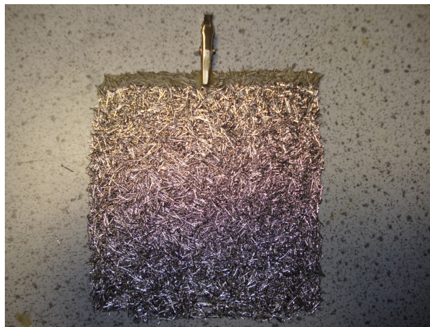
Figure 13: Example of a 100 \times 100\text{ mm} titanium Fibretech electrode, with electrical connection.
