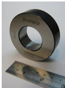
Figure 3.14 Calibrated standard used to evaluate the measurement uncertainty for the multi cross-section workpieces.
