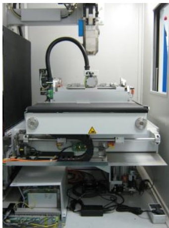
(a) Full internal layout of the CT system.
