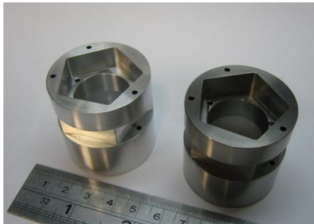
Figure 3.10 Photograph of the multi cross-section workpieces, ruler for scale.
