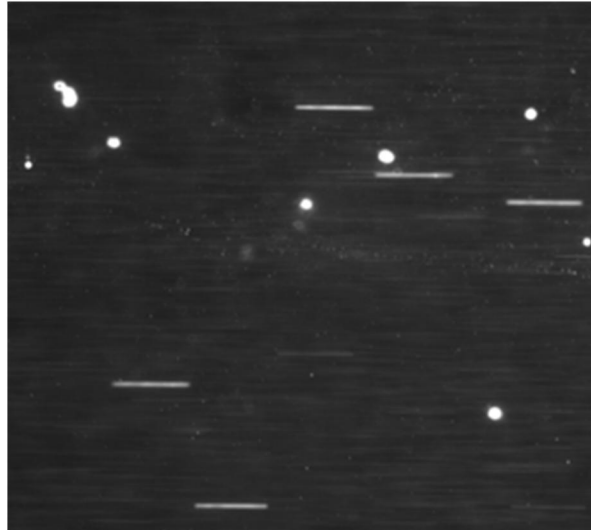
Figure 4-31 An example image of the 10 \mu\text{m} beads in the fluid channel. By comparing the streak lengths when the power is turned on and turned off it is possible to show the effects of ultrasonic excitation across the device. Streak lengths are approximately 200 \mu\text{m} .
