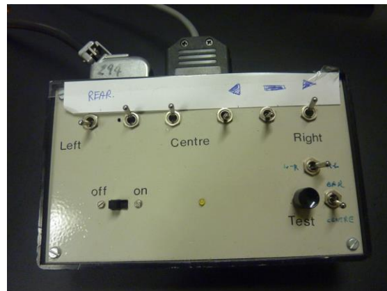
Figure 16 – Light box switch system controlling the cue to turn.
