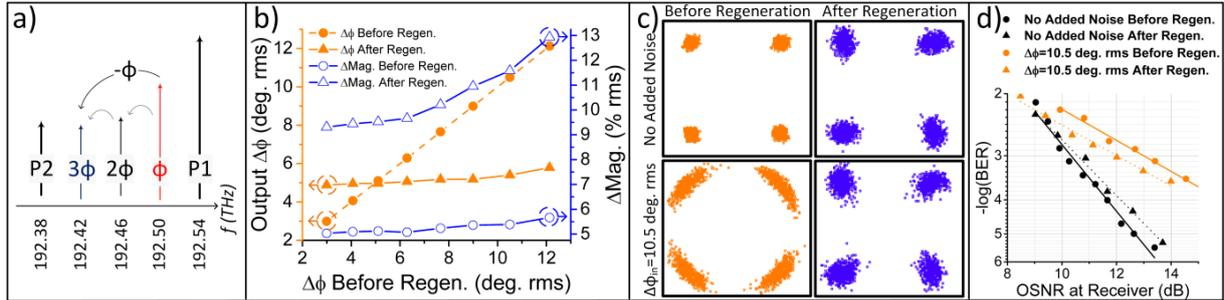
**Fig. 1** a) Wavelength converting, idler-free scheme; b) Phase and magnitude noise before and after regeneration versus input phase noise; c) Constellation plots before and after regeneration for two different noise levels; d) BER before and after regeneration both without additional phase noise and with 10.5 deg. rms phase noise.
