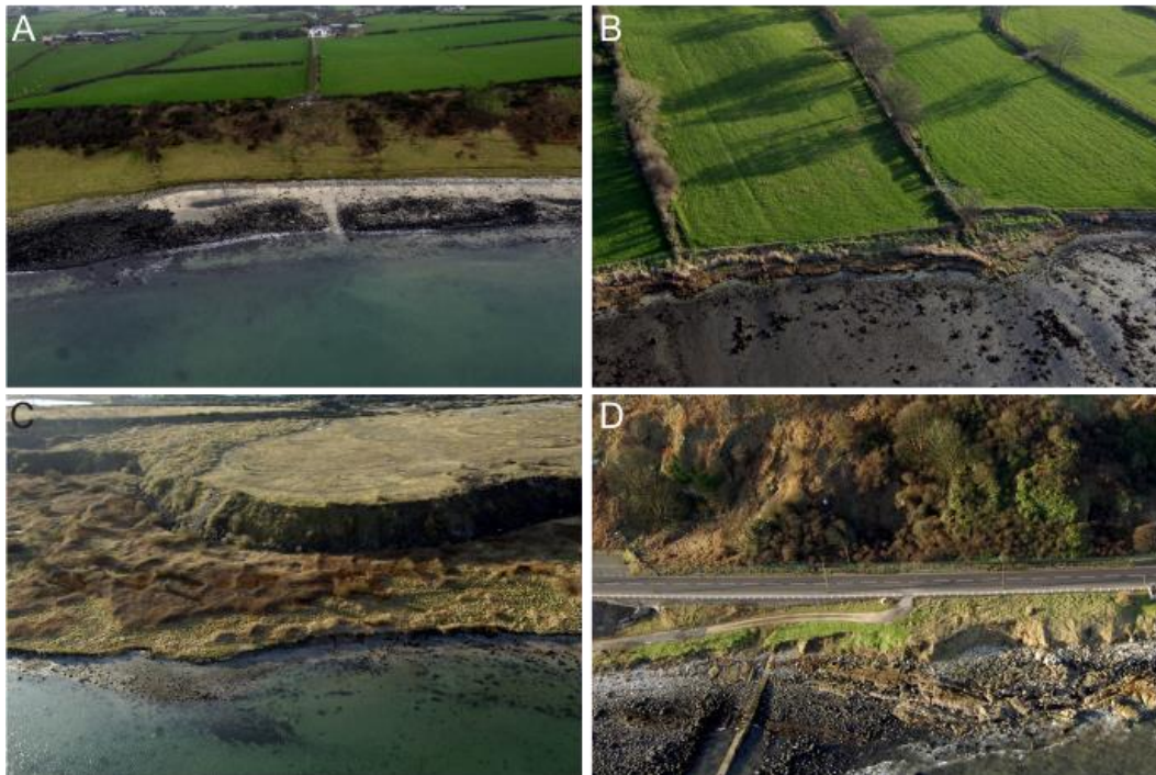
Figure 7. Simplified erosion summary for Larne. Place names are in italics. Black dots show locations of representative coastal erosion visible on the APs. A) Eroding scarp behind beach. B) Possible marsh retreat. C) and D) Eroding scarp behind beach. The simpler erosion by photo layer is used as a proxy of erosion location because the digitized geomorphological/erosion polygons are difficult to see at this scale.
