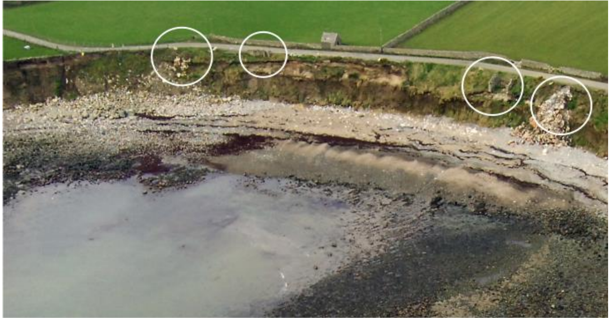
Figure 6. Collapse of historic buildings (circled) at Derryoge due to cliff erosion.
