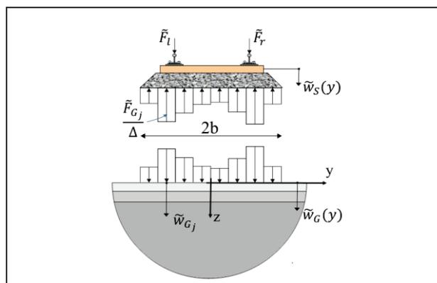
Figure 4. Assumed interface conditions and discretisation of the stress field across the track-soil interface.
