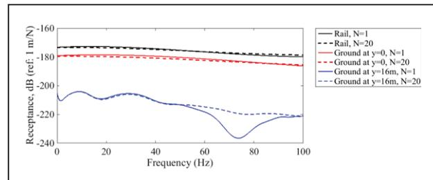
Figure 6. Receptance magnitude at  $y=0$  and  $y=16$  m.
