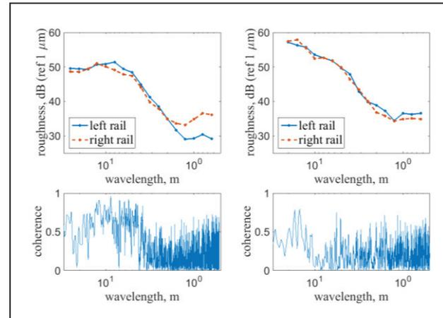
Figure 1. Unevenness spectrum of left and right rail in one third octave bands (top) and coherence function (bottom) for a ballasted (left) and a slab track (right).
