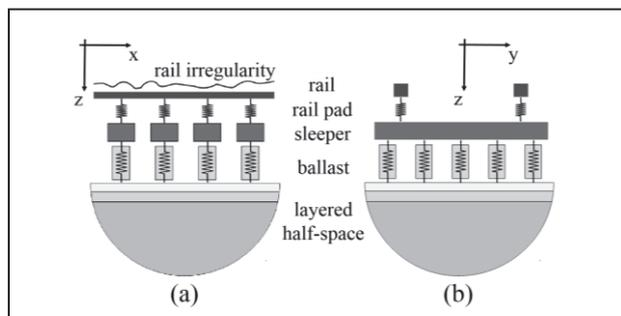
Figure 3. Longitudinal (a) and lateral (b) discretization of the track.
