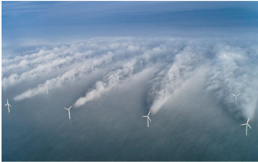
Figure 1.10: Turbulent wakes visualised by “mixing fog” (Emeis, 2010) in the lee of wind energy generators at Horns Rev wind farm, Denmark. Source 1
