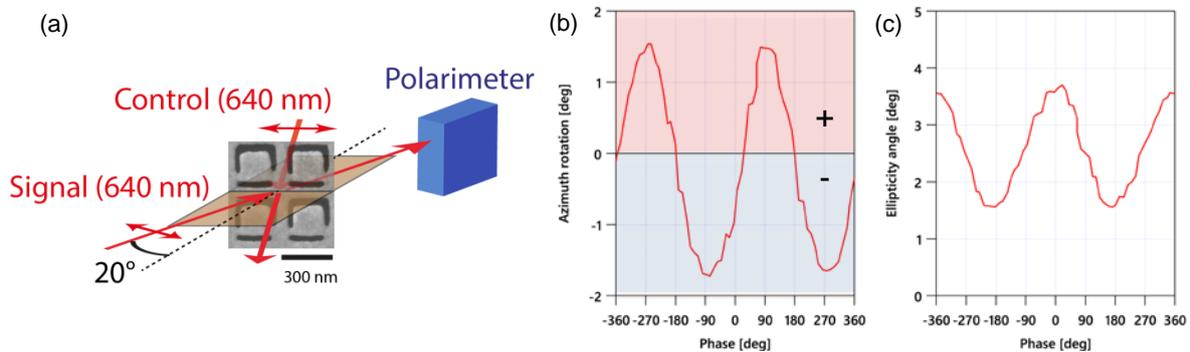
**Fig. 1:** Coherent control of polarization of light with light. (a) Extrinsic 3D-chiral experimental arrangement consisting of metasurface and incident beams that cannot be superimposed with their mirror image. Optical activity in terms of (b) polarization azimuth rotation and (c) ellipticity angle of the output signal beam as a function of the mutual phase of the input beams.
