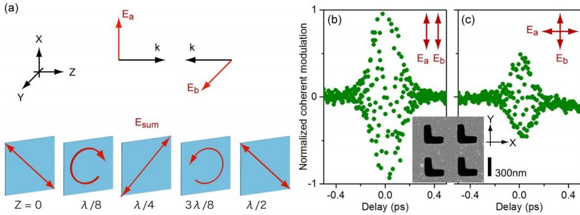
**Fig. 1** (a) Polarization standing wave formed by counter-propagating orthogonally linear polarized beams. (b-c) Normalized coherent absorption modulation as a function of counter-propagating pulse delay for a gold *L*-slot array metamaterial [a section of which is shown in the inset electron microscope image] in intensity (b) and polarization (c) standing waves.
