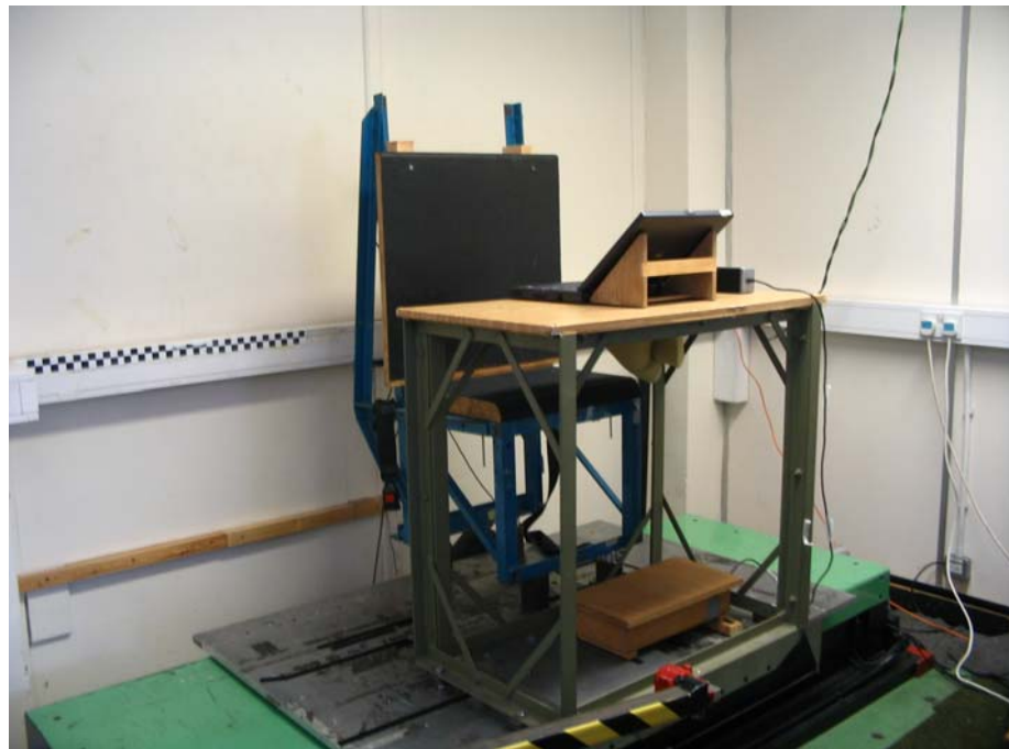
Figure 1 Experimental apparatus for lateral excitation.
