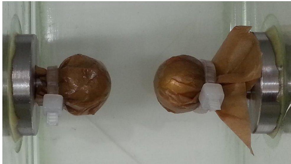
Figure 3:2 Covered electrode system with tight bonded paper kraft
