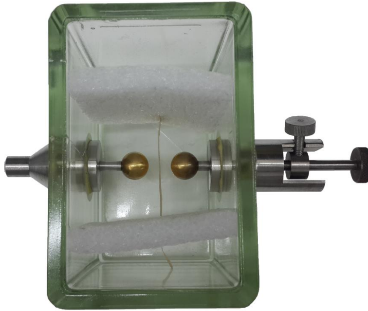
Figure 3:3 Sample holding tank for paper barrier test
