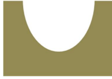
Figure 3-3: Schematic profile of a laser ablated channel which is parabolic.
