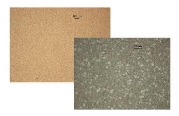
Figure 106: Optical image of CuSbSx deposited at 240  $^{\circ}$ C at different magnifications. The film thickness was 800 nm.
