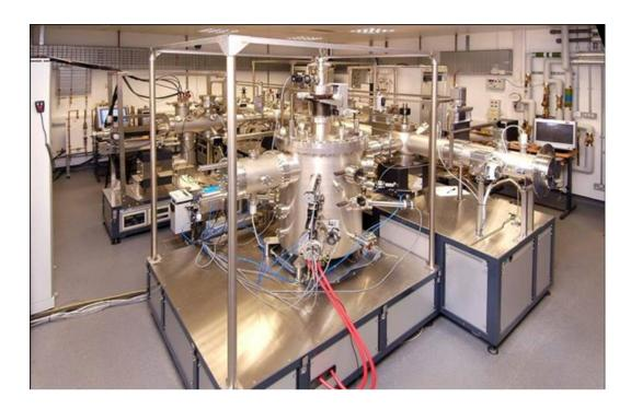
Figure 13: High throughput UHV PVD system in surface science group in chemistry [27]
