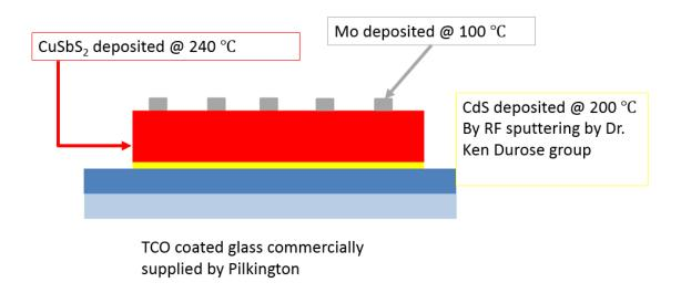
Figure 93: CuSbS<sub>2</sub> solar cell fabricated by single stage method
