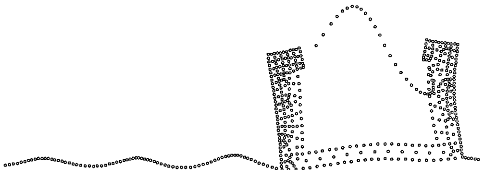
Figure 18. Displaced shape plot of part of the model at 37 Hz.
