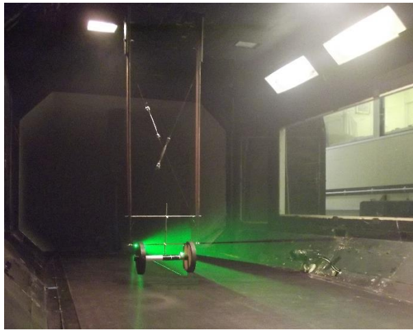
Figure 5.17: Front view of the PIV experimental setup of isolated wheelset case
