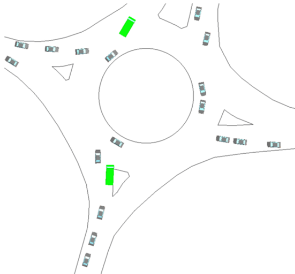
Figure 2-7 Example microscopic simulation model set up to show a car entering from nearside lane alongside another circulating in inner lane, while a heavy vehicle waits in the offside lane of the bottom arm.
