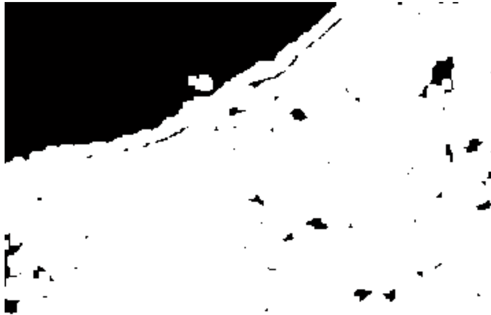
Figure 5-23 : The result after morphological dilation.
