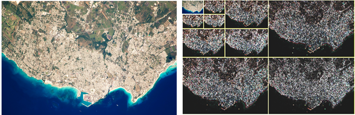
Figure 6-4 : Three level decomposition of an example satellite image. Left hand side is the original image, right hand side demonstrates the three level decomposition.
