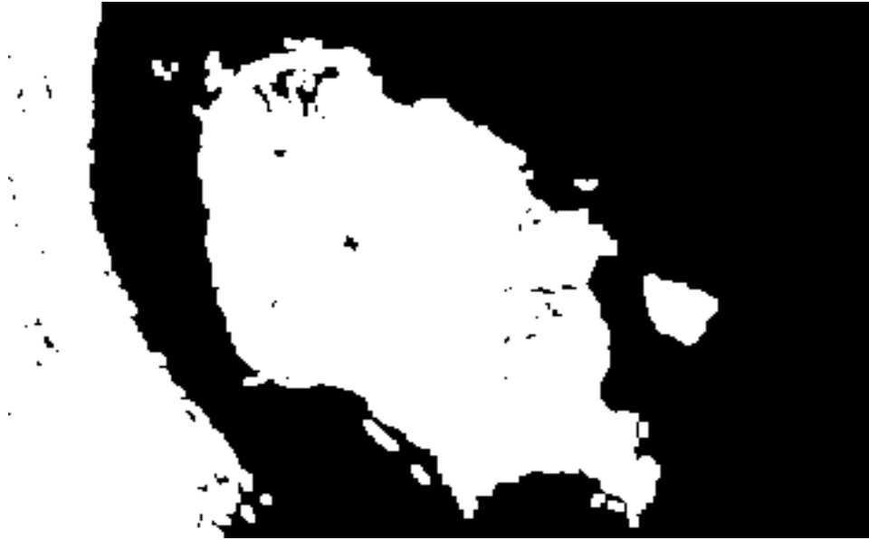
Figure 5-5 : The image after dilation using a square structure element has been performed.
