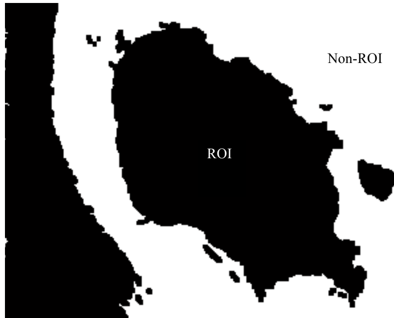
Figure 5-6 : The image is processed by filling of regions and holes.
