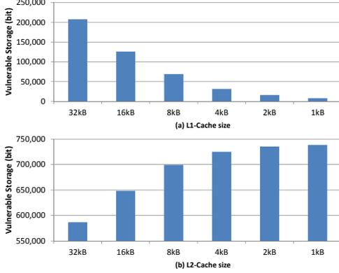
Fig. 7. The impact of L1-Cache resizing on (a) L1-Cache and (b) L2-Cache vulnerabilities
