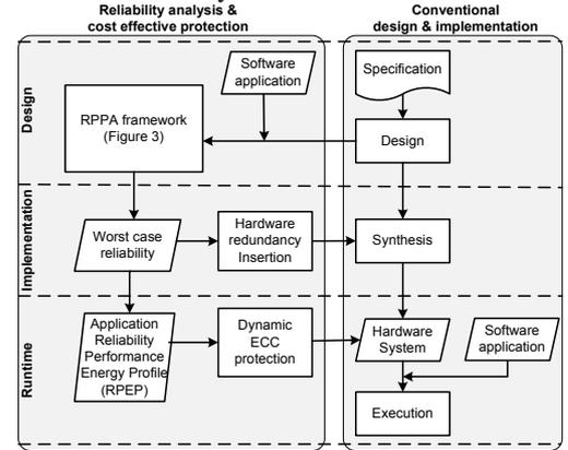
Fig. 9. Proposed reliable design flow
