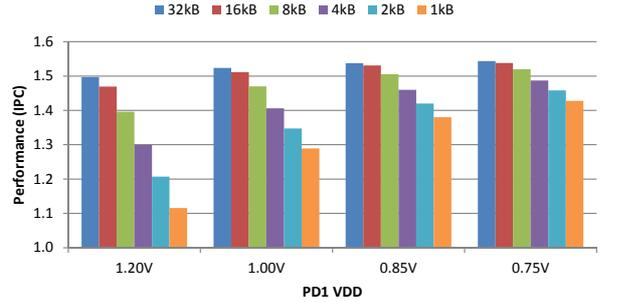
Fig. 11. The impact of L1-Cache resizing on performance under VFS
