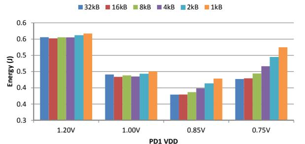
Fig. 12. The impact of L1-Cache resizing on energy under VFS
