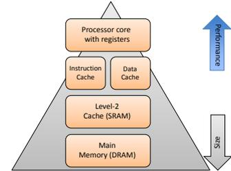
Fig. 1. Microprocessor memory hierarchy
