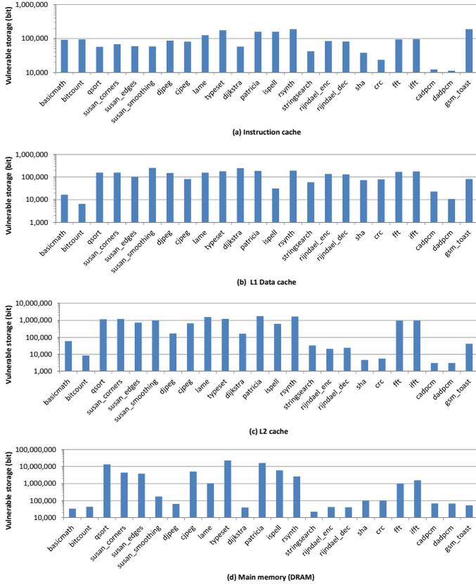
Fig. 5. Vulnerable storage of different memory components for different MiBench benchmark applications: (a) L1 instruction cache (I-Cache), (b) L1 data cache (D-Cache), (c) L2-Cache and (d) DRAM
