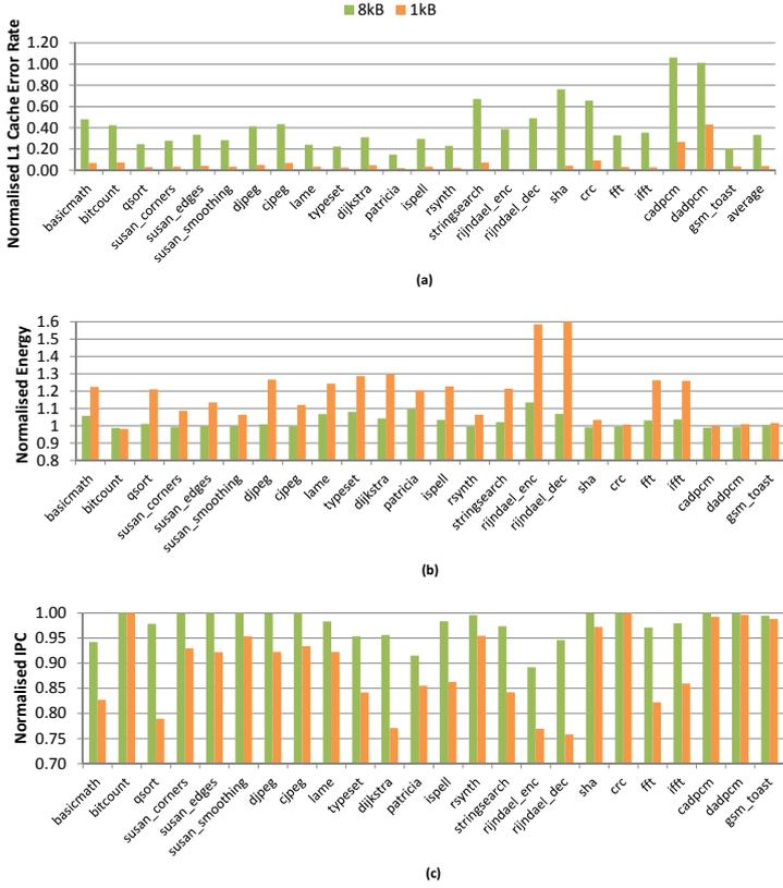
Fig. 13. The impact of L1-Cache resizing on (a) L1-Cache reliability (b) performance and (c) energy; under supply voltage of 0.85V
