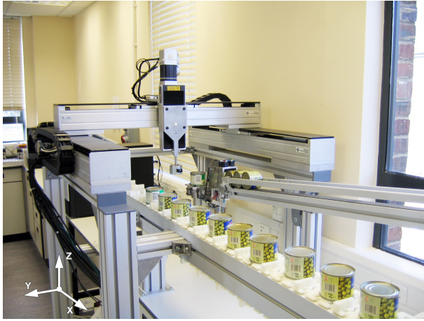
Fig. 8 The gantry robot with the three axes marked.
