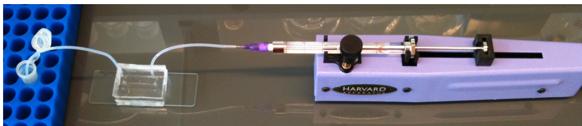
Figure 5.4 Microfluidic device designed for transcription from a DNA-containing H_{II} phase. Transcription assay components are fed into the device from a Harvard NanoMite syringe pump at a rate of 0.5 \mu\text{L}/\text{min} , with the transcription product and any waste consumables collected in a microcentrifuge tube, ready for purification.
