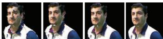
Figure 60: From left to right a) Raw SDCT reconstruction, b) Output of CERTH’s previous work [Alexiadis, 2013], c) Output of [Alexiadis, 2013] after applying the proposed weighted smoothing method, d) watertight volumetric reconstruction [Alexiadis, 2014]
