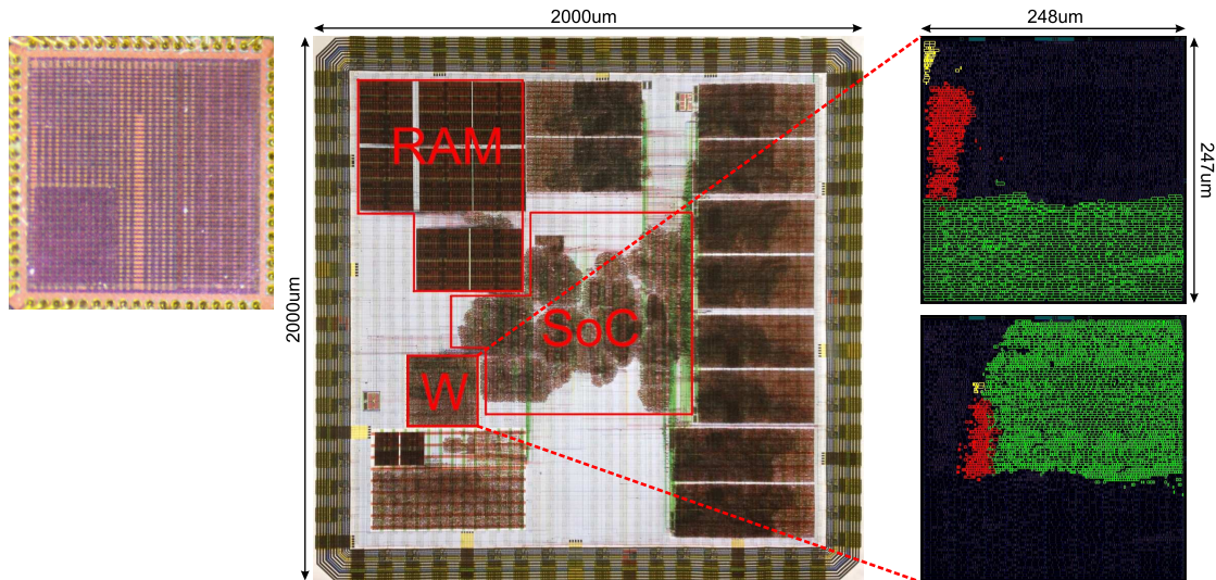
Figure 4.13: The layout (middle), die photo (left) and the hard macro watermark module ('W'), highlighting the watermark circuit (top right) and noise generator (bottom right), integrated in chip I.
