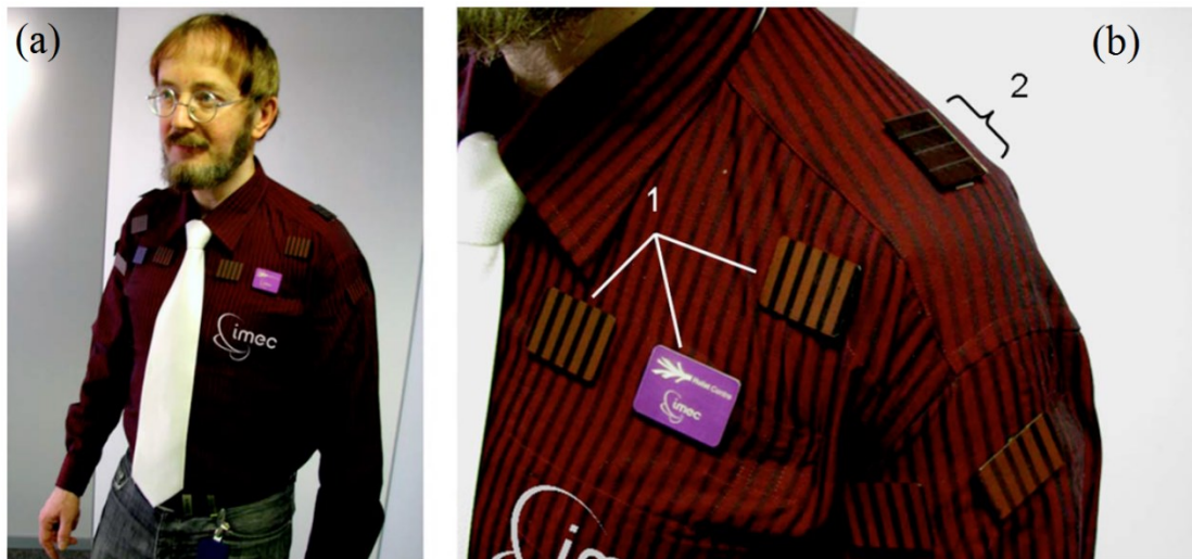
Figure 3.20 (a): Electrocardiography system integrated in a shirt. (b): (1) TE modules and (2) PV cells after Leonov [72]
