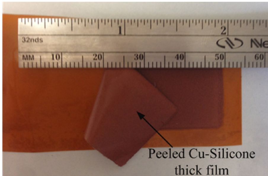
Figure 5.2 Adhesion demonstration of Cu-silicone thick film on Kapton substrate
