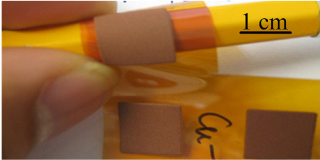
Figure 5.4 Cu-epoxy thick film pattern rolling on a pencil
