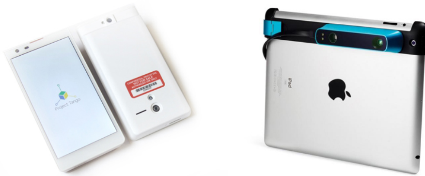
Figure 2.5: Mobile depth sensors. Google Project Tango (left), Structure (right).
