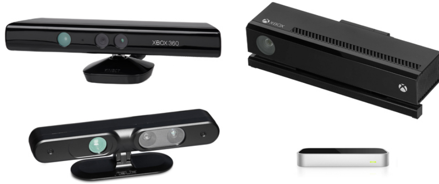
Figure 2.4: Consumer depth sensors. Microsoft Kinect (top left), Microsoft Kinect v2 (top right), Asus Xion Pro (bottom left) and Leap Motion (bottom right).
