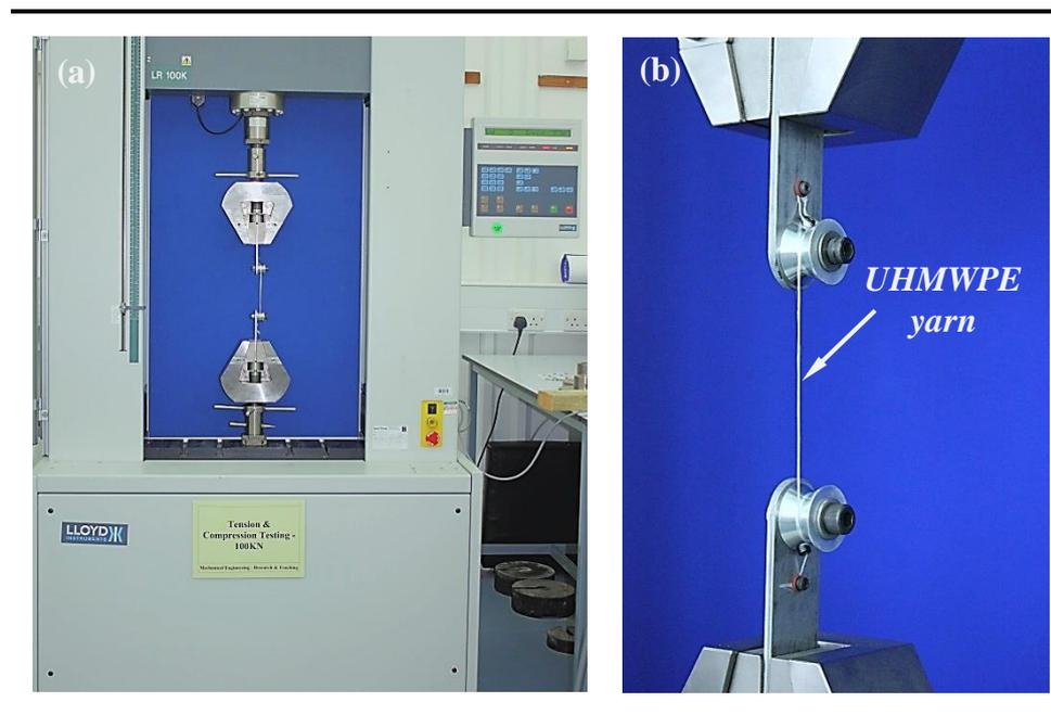
**Figure 3-8. Tensile testing setup (a) and jig assembly (b) for UHMWPE fibres.**
