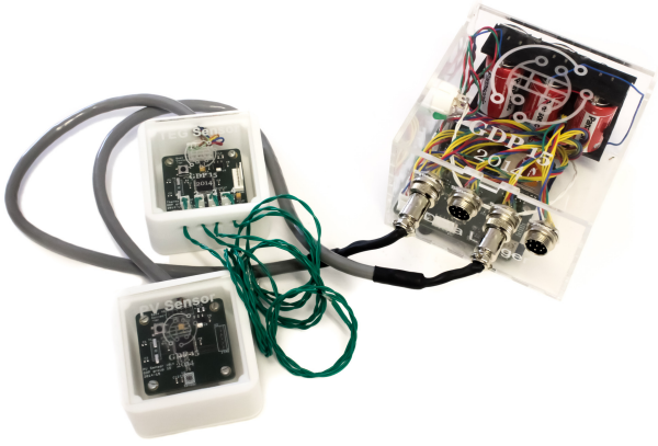
Figure 5: The DCU with two sensor modules (PV and TEG) attached.
