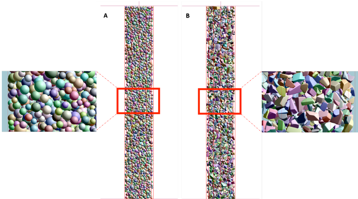
Figure 10. Specimen preparation. a) spheres are randomly distributed in a cylinder b) spheres are replaced by potential particles(DEM ballast)
