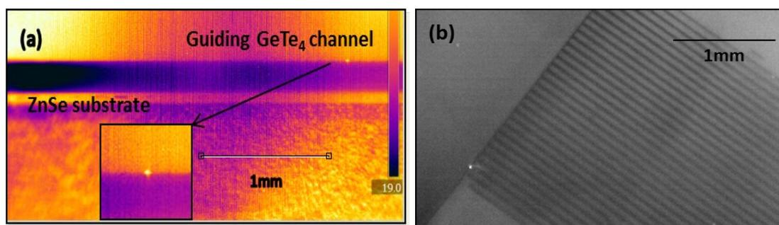
Fig. 1 Infrared images of the output facet of a channel waveguide showing light guidance (a) at a wavelength of  $3.5\ \mu\text{m}$  (cross-sectional view) and (b) at a wavelength of  $6.5\ \mu\text{m}$  (top view)
