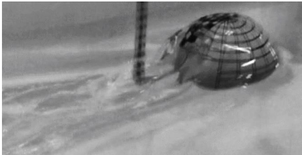
Fig.7 Turbulent wake behind the sphere at Re = 4.4 \times 10^5
