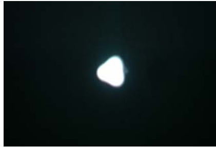
Fig. 3 IR image of the near-field pattern of the spliced bismuth-oxide-based glass HF.
