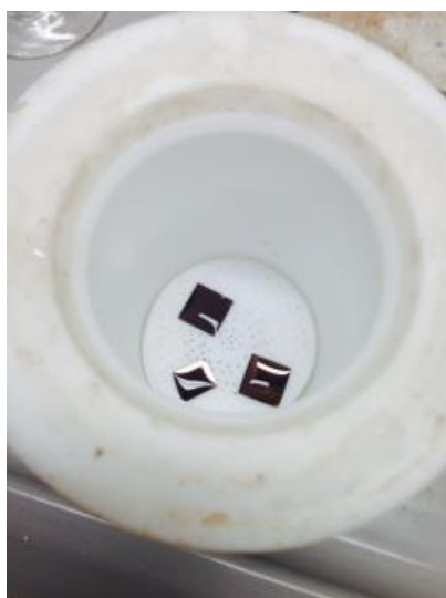
Figure 35 – 3 substrates, each cleaned in different manners, coated in TPAOH ready for SAC
