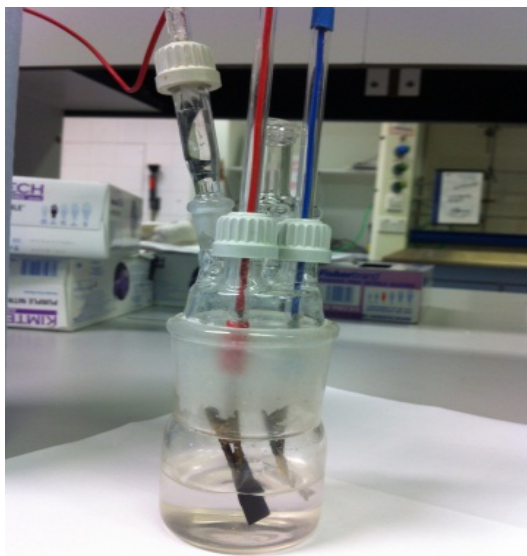
Figure 3.11: Three-electrode cell used for electrochemical processing
