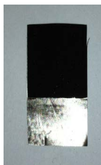
Figure: 3.16: \text{Mn}_3\text{N}_2 ink film over titanium current collector
