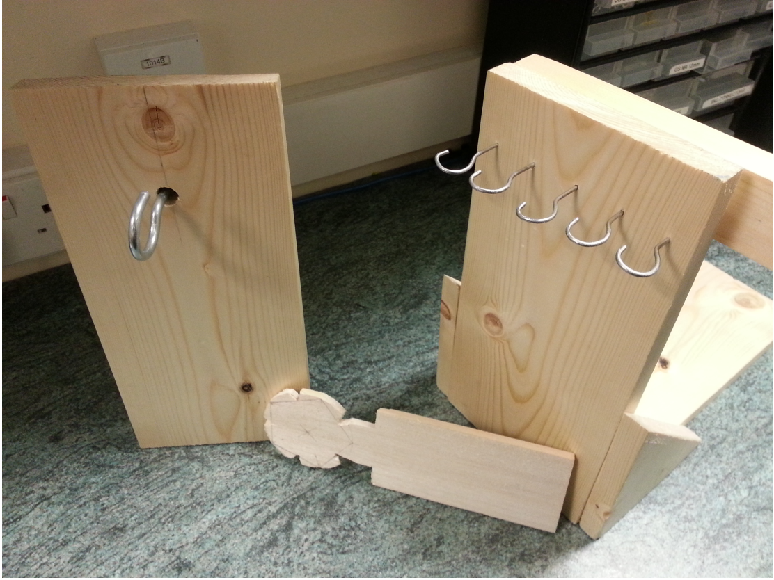
Figure 6.16: The ‘Leonardo’ style rope winding machine used to produce the home-made litz wire. The bracket on the right of the image holds five hooks which turn simultaneously through the use of a crank. The left block holds a large hook which can be fixed in place or allowed to rotate. The separator is visible at the bottom of the image. Based upon[122].
