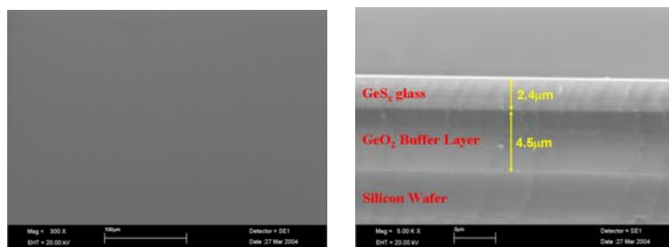
Fig. 2 SEM picture from top view (left) and side view (right) of the germanium sulphide glass film on silicon wafer with \text{GeO}_2 buffer layer
