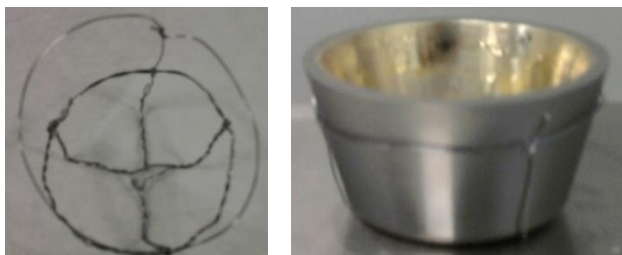
Figure 5.6 Photograph showing (a) basket made by tantalum wire, (b) the tungsten liner with basket
