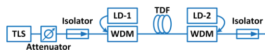
Fig. 1: Experimental setup. TLS: tunable laser source; LD: laser diode; WDM: wavelength division multiplexer; TDF: thulium-doped fiber.
