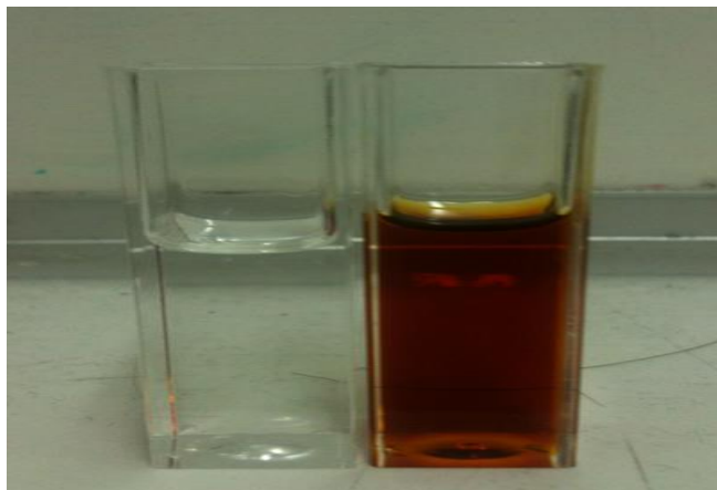
Figure 3-5 The two types of mineral oil used in this work, the left one is the fresh oil and the right one is the service aged oil.
