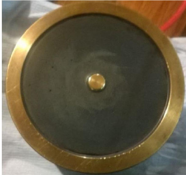
Figure 3-1 Top electrode of the new PEA system
