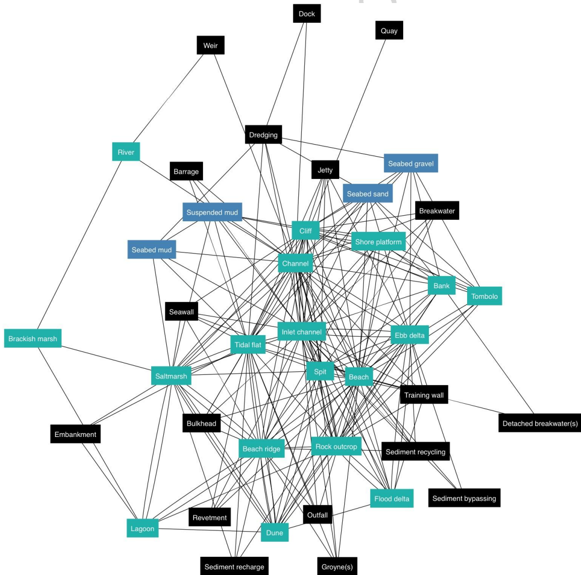
Figure 4 – Functional interactions between landforms and human interventions for components summarised in Tables 1 and 2 (hinterland omitted). Landforms are in green, human interventions in black and sediment stores in blue. Note that this diagram is not
