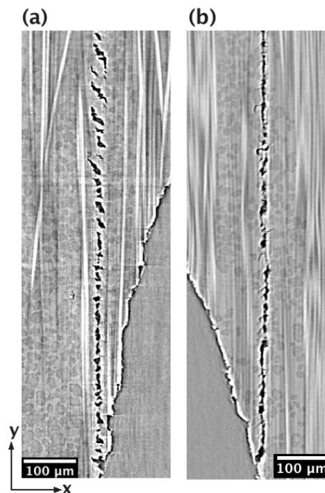
Figure 4. 11 – Comparison of the micromechanical behaviour along the 0^\circ ply split in (a) quasi-static case loaded to 60% UTS, and (b) fatigue loaded to 50% UTS with number of cycles of 10^4 .
