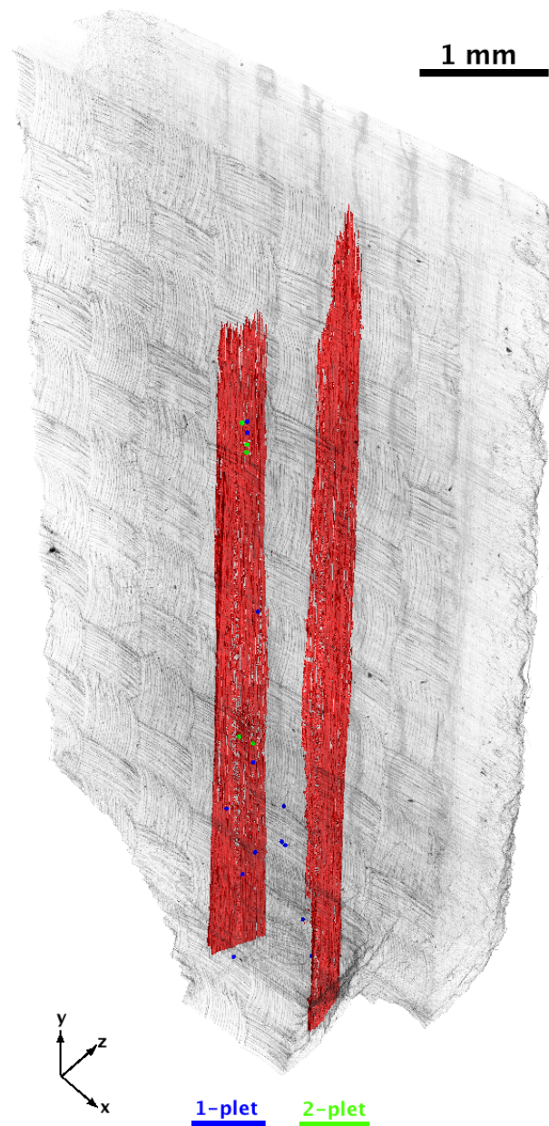
Figure B. 1 - Fibre failure distribution in the bulk composite for the 50% UTS and 10^5 cycles considering the entire damaged volume.
