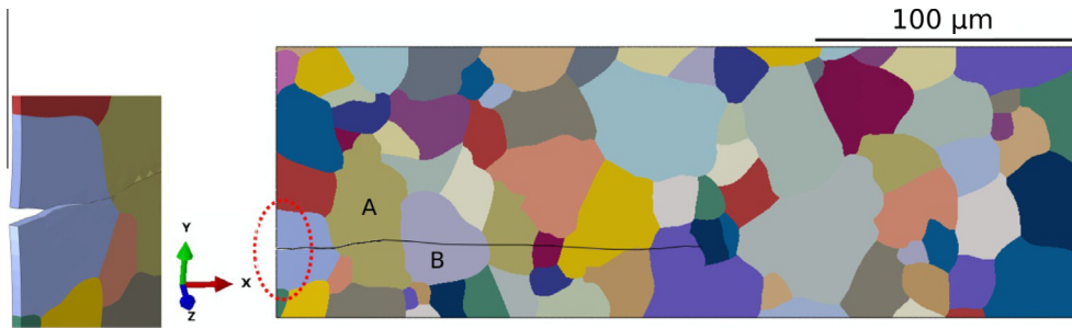
Fig. 16. Short crack growth path in pseudo-3D model predicted from XFEM (crack growth length 163.8 \mu\text{m} ).
