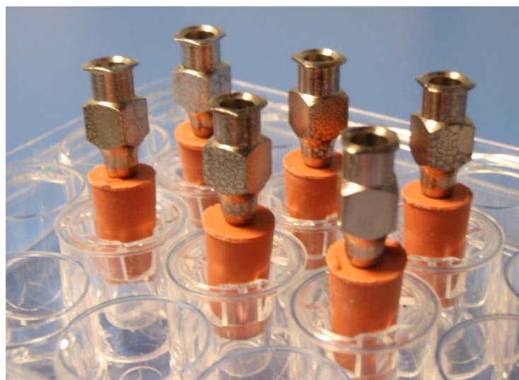
Figure 2-15 Multiple bungs inserted into transwell plate for simultaneous pressurisation of multiple transwells.
