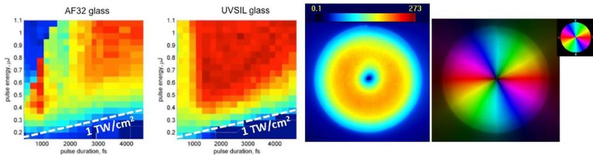
**Fig. 1** Retardance as a function of pulse duration and energy measured for borosilicate glass AF32 and silica glass UVSIL. Quantitative birefringence measurements of 100  $\mu\text{m}$  diameter converter imprinted in the bulk of AF32 glass.
