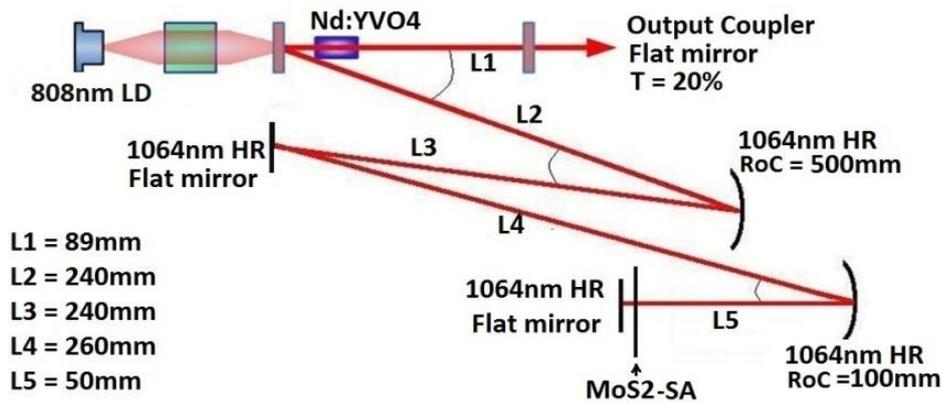
Fig 2. The schematic diagram of laser, HR-High reflection, T-Transmission ratio, RoC – Radius of Curvature of the mirror.
