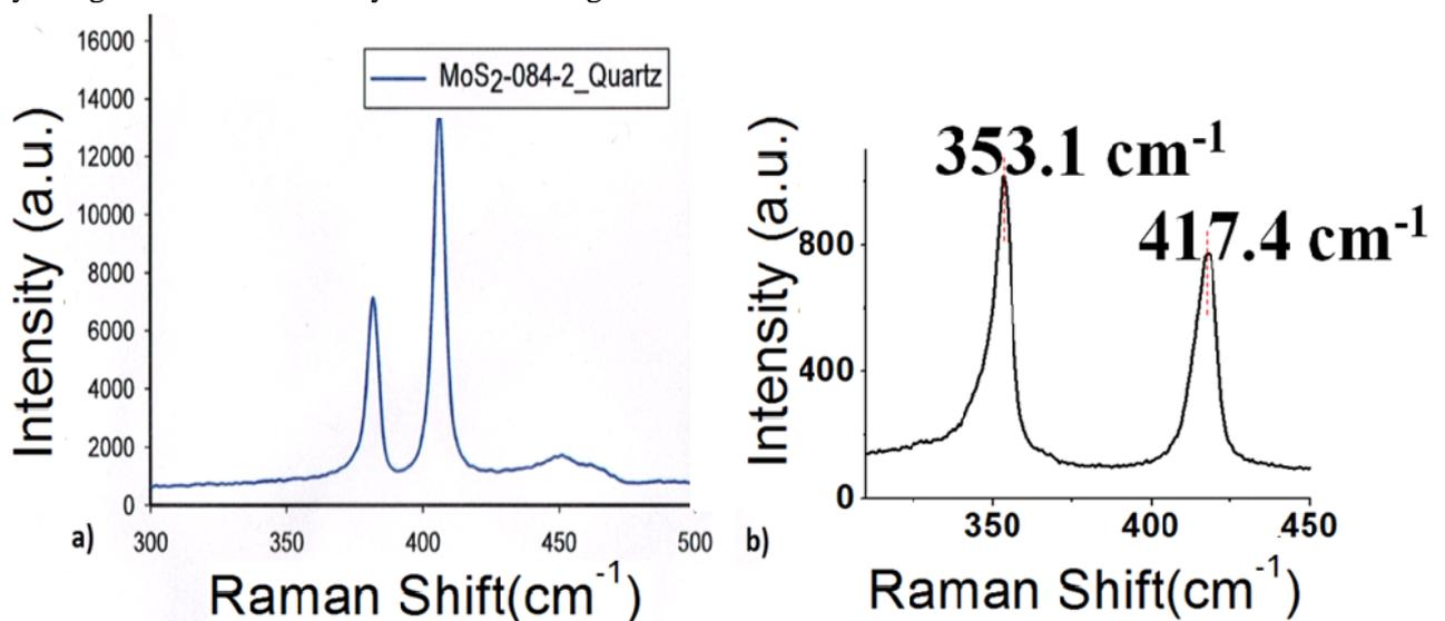
Fig. 1 Raman spectrum of (a)  $\text{MoS}_2$ -SA (b)  $\text{WS}_2$ -SA sample.
