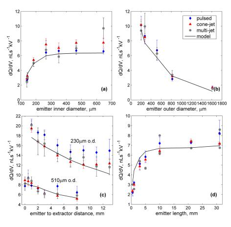
FIG. 3. (a)–(d)  $\left\{\frac{dQ}{dV}\right\}$  variation with geometry within pulsation, cone-jet and multi-jet modes, for different geometry changes.
