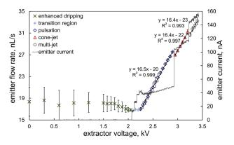
FIG. 1. Variation of flow rate with voltage across the four major regimes of electrospray. NaI doped PC, emitter i.d.-o.d. =  $125-230 \mu m$ .
