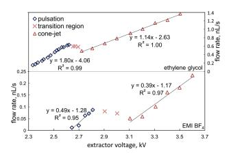
FIG. 2. Variation of flow rate across pulsation and cone-jet mode, for NaI-doped EG and EMI BF<sub>4</sub>.
