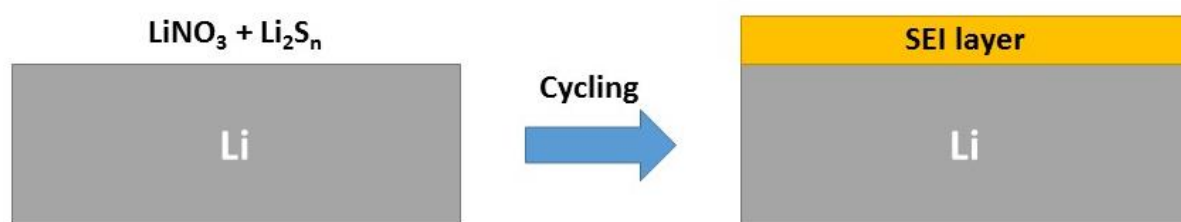
Figure 7.1 Illustration of the formation of SEI layer on Li metal in the Li-S battery.
