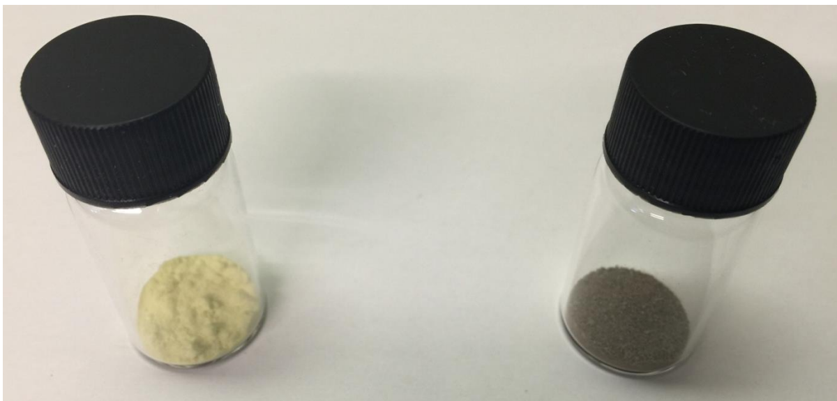
Figure A 7 Sulfur powders before (left) and after (right) heating treatment.
