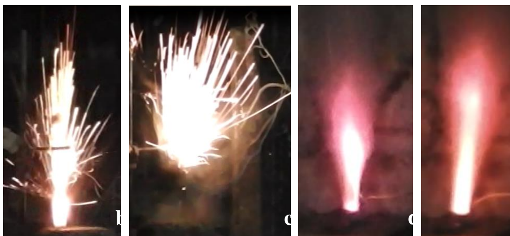
Figure 3.4.1 - Initial Burn Test Results a) Safety Test \text{NaNO}_3 , b) Safety Test \text{CsNO}_3 , c) Pressed Burn Test \text{CsNO}_3 and Pressed Burn Test \text{KNO}_3
