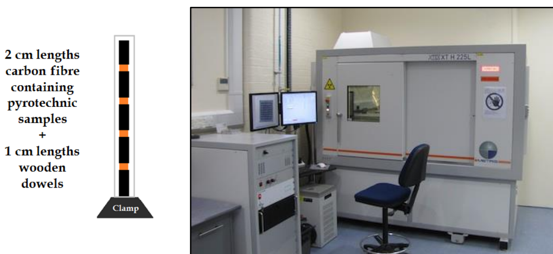
Figure 2.2.1 - Pyrotechnic Sample Set-up and X-Tek-HMX CT equipment 2
