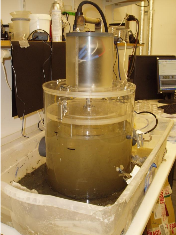
Figure 4.6 Annular mini flume at Southampton Oceanography Centre used to assess critical shear velocities of sediments.
