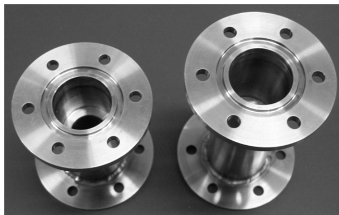
Figure 9-2: Catalyst beds 1 (Left) and 2 (Right), central temperature measurement standpipe not shown
