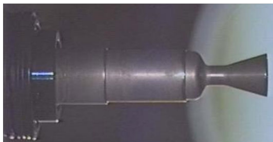
Figure 9-7: ECAPS HGHP 1N thruster [99]
