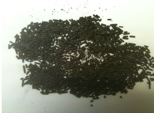
Figure 9-31: MnOx-Ce/U-3 after runs 23-26
