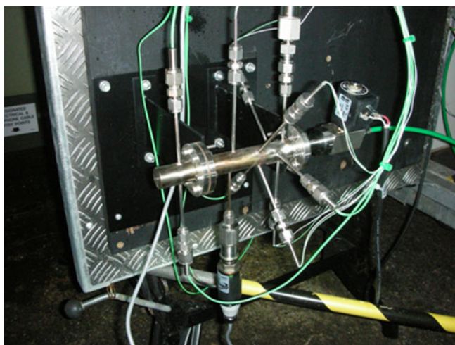
Figure 2. Test stand and instrumented catalyst bed
